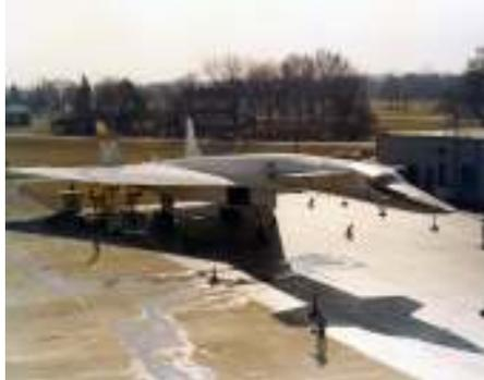
It is powered by six General Electric YJ93-GE-3 turbojet engines which were rated at 22,000 pounds of thrust. The maximum speed achieved was Mach 3.1. XB-70A Valkyrie 62-0001 is in the collection of the National Museum of the United States Air Force.
