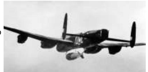
The Grand Slam bomb was 26 feet, 6 inches and had a maximum diameter of 3 feet, 6 inches. When fully loaded with the explosive material, Torpex, the bomb weighed 22,000 pounds. The bomb case was cast of steel at the Clyde Alloy and Steel Company, Glasgow, Scotland, then, after several days of cooling, machined to its precise shape. The casing made up approximately 60% of the bomb's total weight. The bomb case was filled with molten Torpex.
